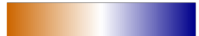
Figure 3.35: A quasi-continuous colour palette derived by interpolating between the colours darkorange3 , white and darkblue .
