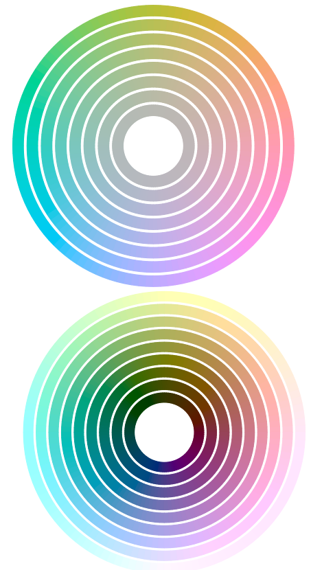
Figure 3.37: Circles in HCL colorspace. Upper panel: The luminosity L is fixed to 75, while the angular coordinate H (hue) varies from 0 to 360 and the radial coordinate C = 0, 10, \dots, 60 . Lower panel: constant chroma C = 50 , H as above, and varying luminosity L = 10, 20, \dots, 90 .
